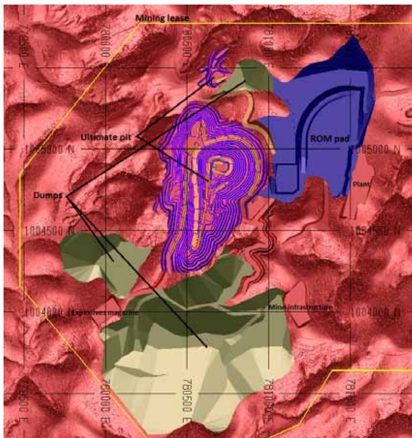
Figure 5.2 Final pit design and infrastructure layout
