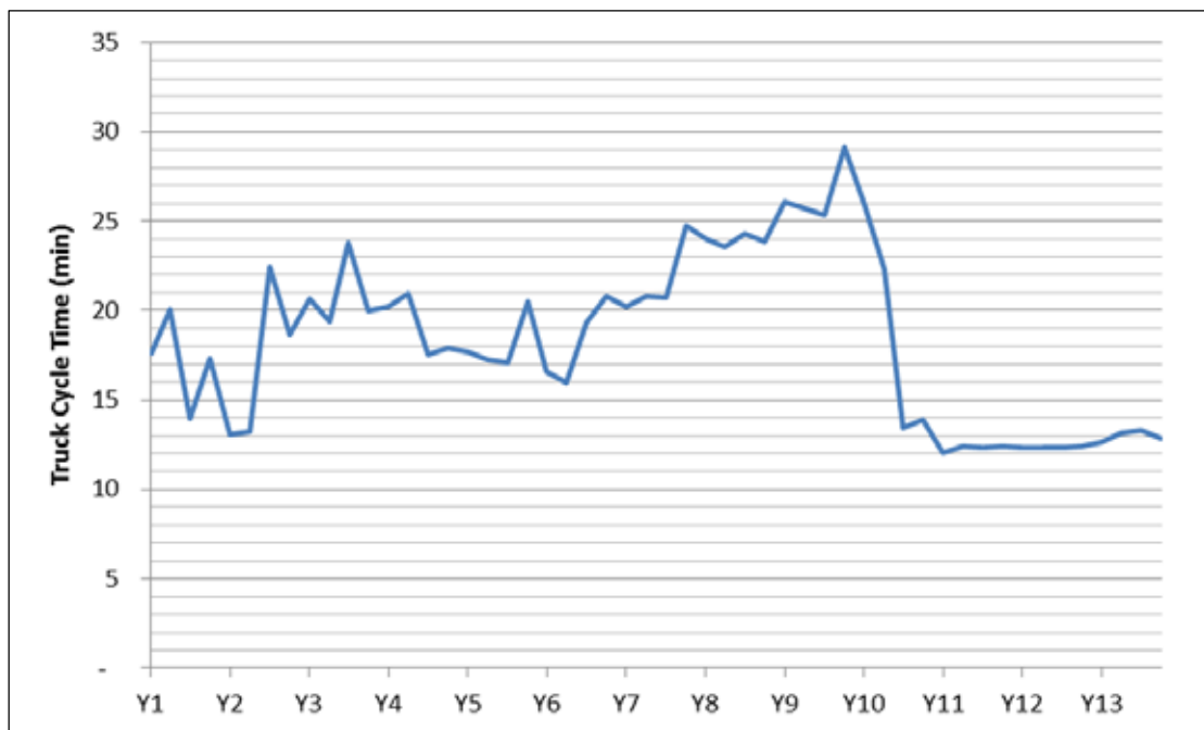
Figure 5.57 Average cycle times for dump trucks
