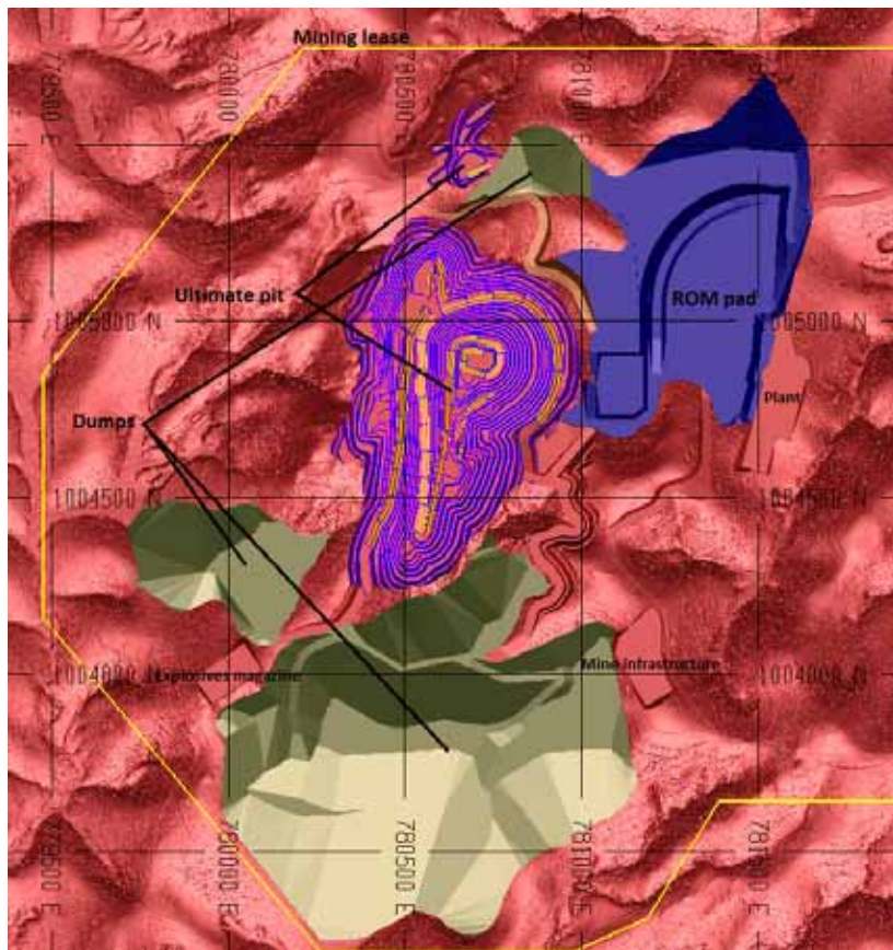
Figure 1-2: Final pit design and infrastructure layout
